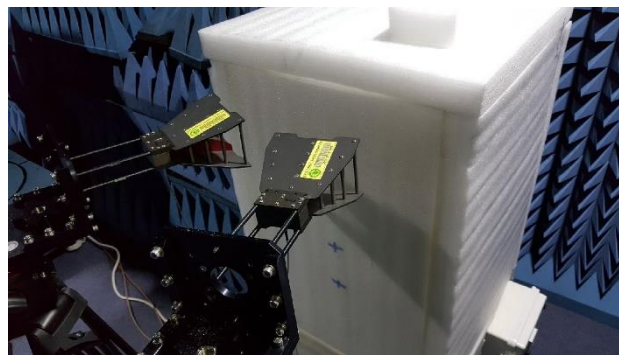
Fig 5. Measurement set-up with non-reflective temperature and humidity chamber.
