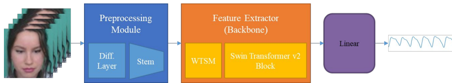
Figure 1. Overall architecture for remote heart rate estimation
